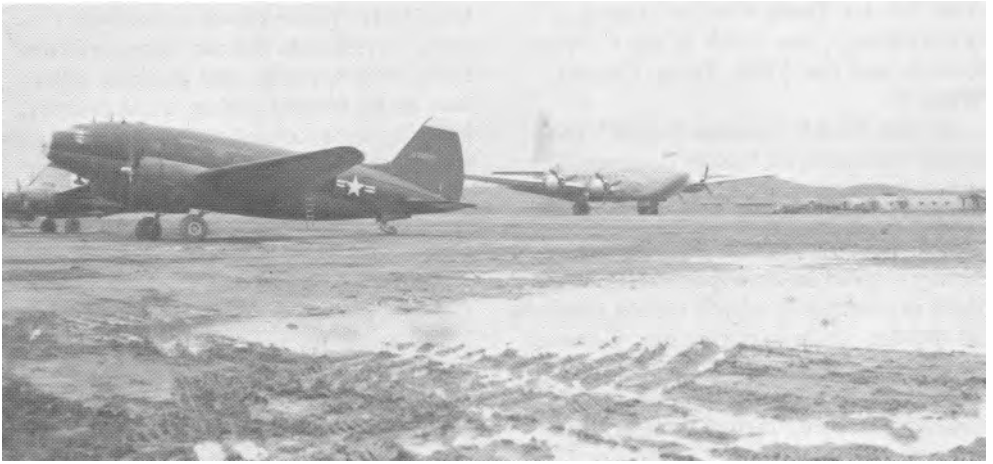
Cargo aircraft like the C-124 Globemaster (rear) and the C-46 Commando airlifted tons of war supplies.
