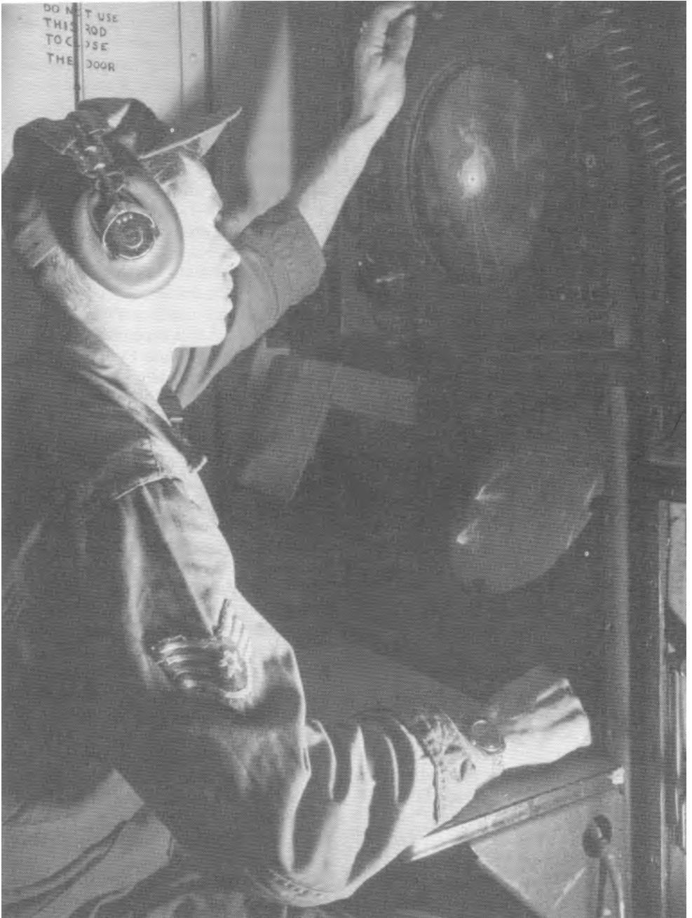
Ground Control Approach Units like this one track aircraft and assist pilots making instrument landings in bad weather.
