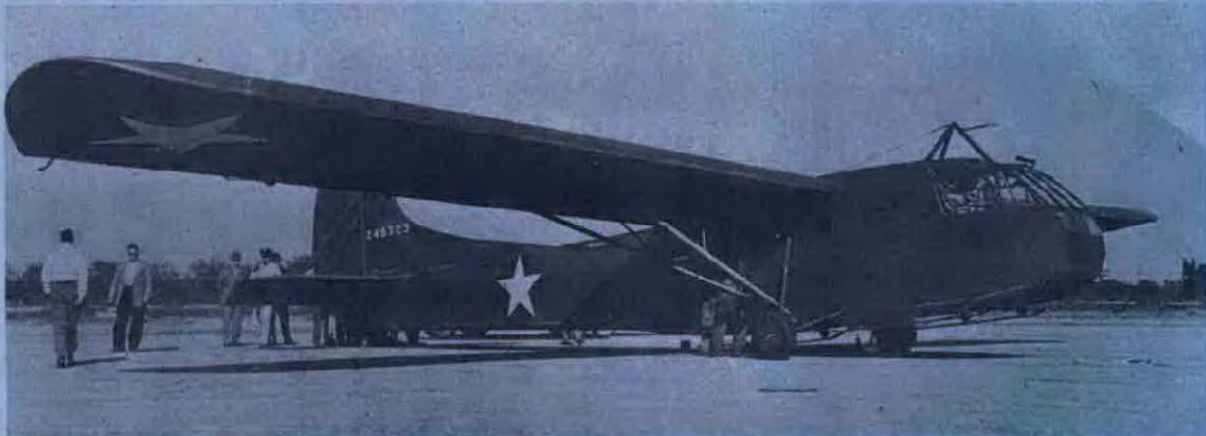
CG-4A combat glider. Glider carries thirteen fully equipped troops, glider pilot, and copilot.
