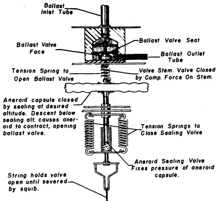
Figure 10. Automatic ballast valve.
