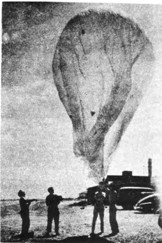
Figure 12: Neoprene balloon encased in a nylon shroud
