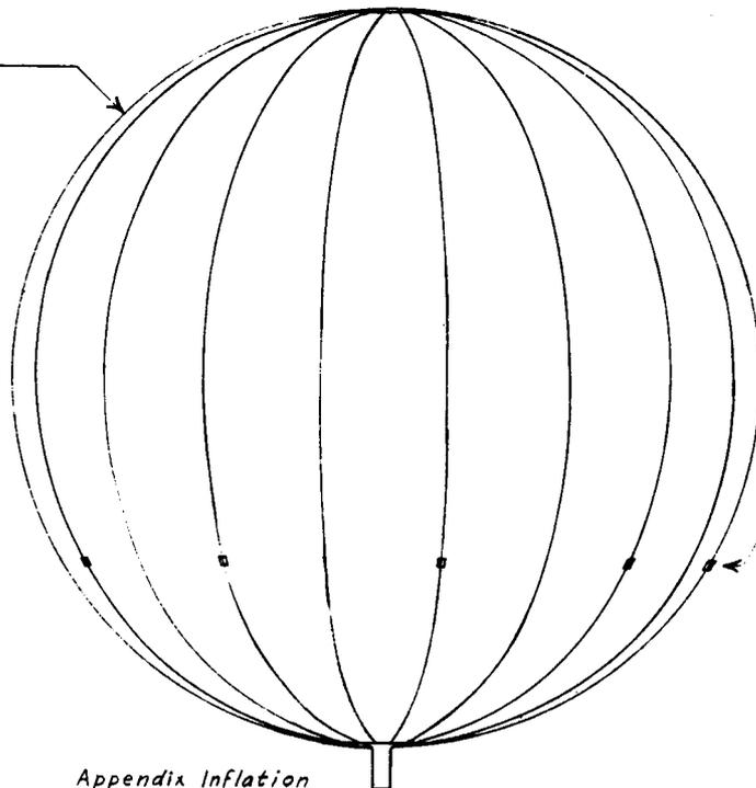
9 eyelets in reinforced seams for attaching bridle rigging to balloon at 30° below balloon's equator.
