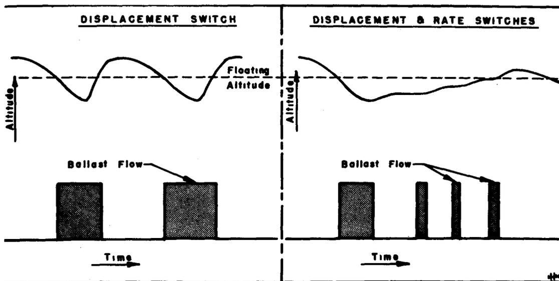
Figure 13. Height-time curve, showing ballast control action.
