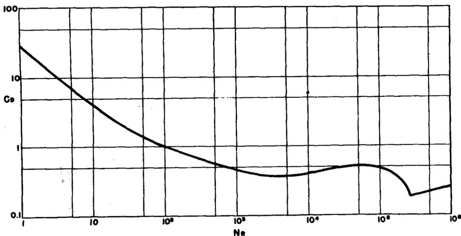
Figure 27. Drag coefficient vs. Reynolds Number, for sphere.
