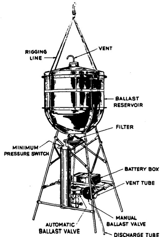
FIG. 3. Ballast-release assembly.
