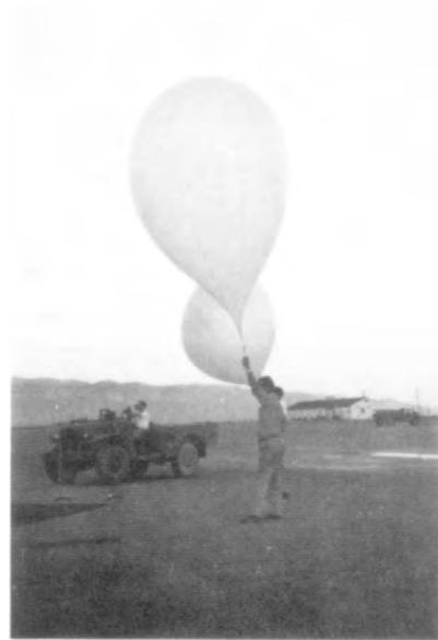
**Launch of Project MOGUL neoprene balloons, Alamogordo AAF, NM, June 1947.** While awaiting the experimental polyethylene balloons, NYU engineers utilized long trains of the smaller neoprene balloons as a stopgap method of placing their acoustic sensors in the upper atmosphere. These balloon trains consisted of a variety of equipment and measured more than 600 feet long (*see Atch 25*). *Photo Collection of Albert P. Crary.*
