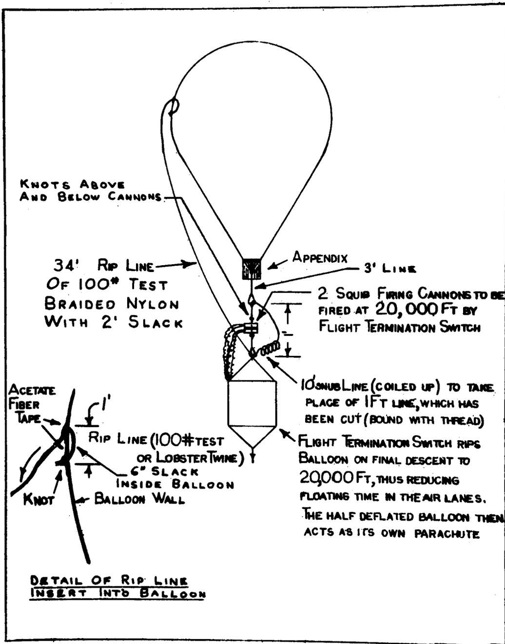
Figure 14: Rip-out line in place on balloon
