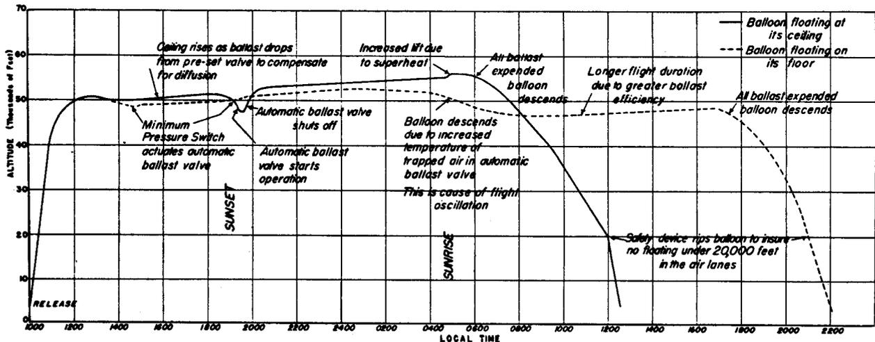
FIG. 6. Idealized time-altitude curves for various balloon-control systems.
