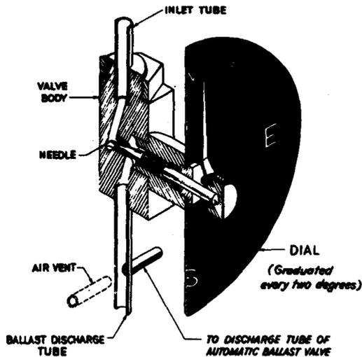
Figure 9. Manual ballast valve.
